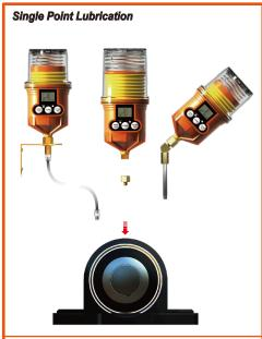
Direct Straight/Angle Mount (with or without extension tube) is always preferable. However, for applications not allowing any direct mounts or extension mounts, remotely mount the unit using a 6mm O.D. (1/4") pre-filled lube line.
